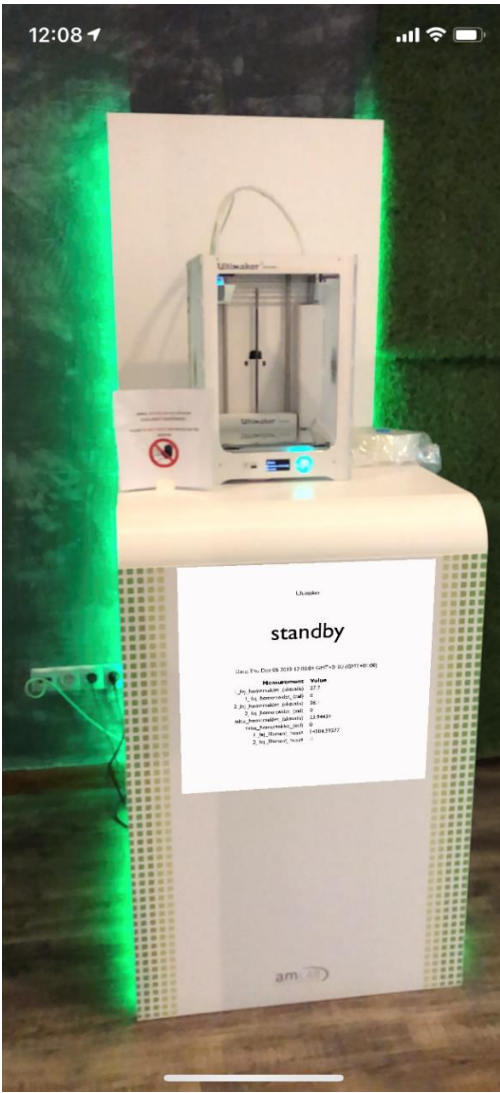
Figure 38: The application developed by PBN (Am-LAB) staff shows the data of the 3D printer using Augmented Reality
